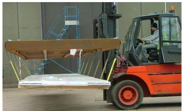
In all cases of **handling** and storage, it is important to prevent the panels from being scratched by friction during operations.
