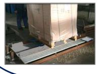
**Strength test :** we carried out specific tests on a test bed and we did not notice any residual deflection nor any visible damage.
