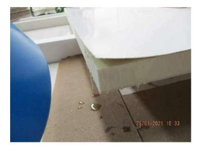
5. Once the mixture has been applied, take 2 pieces of panels or boards and place them above and below the panel to protect it from the clamps.
