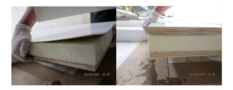
6. Put on a first clamp and do not remove the excess resin as shown in the photo below
