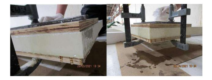
7. Remove the excess of resin from the panel core with the spatula
