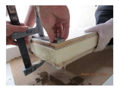
Put a second clamp in order to have 2 on the edges of the panel, tighten.
