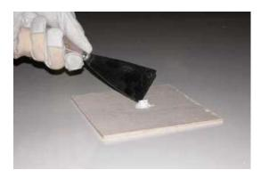
4. Apply the mixed gelcoat on the damaged area, and lay polyester film over the area, then level the film and gelcoat out with a flat scraper.
