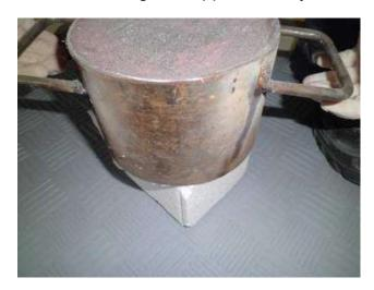
12. After good polymerization (after several hours), remove carefully the mold
