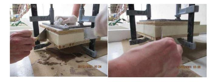
Once the resin has hardened (After about 1 hour), remove the clamps.
